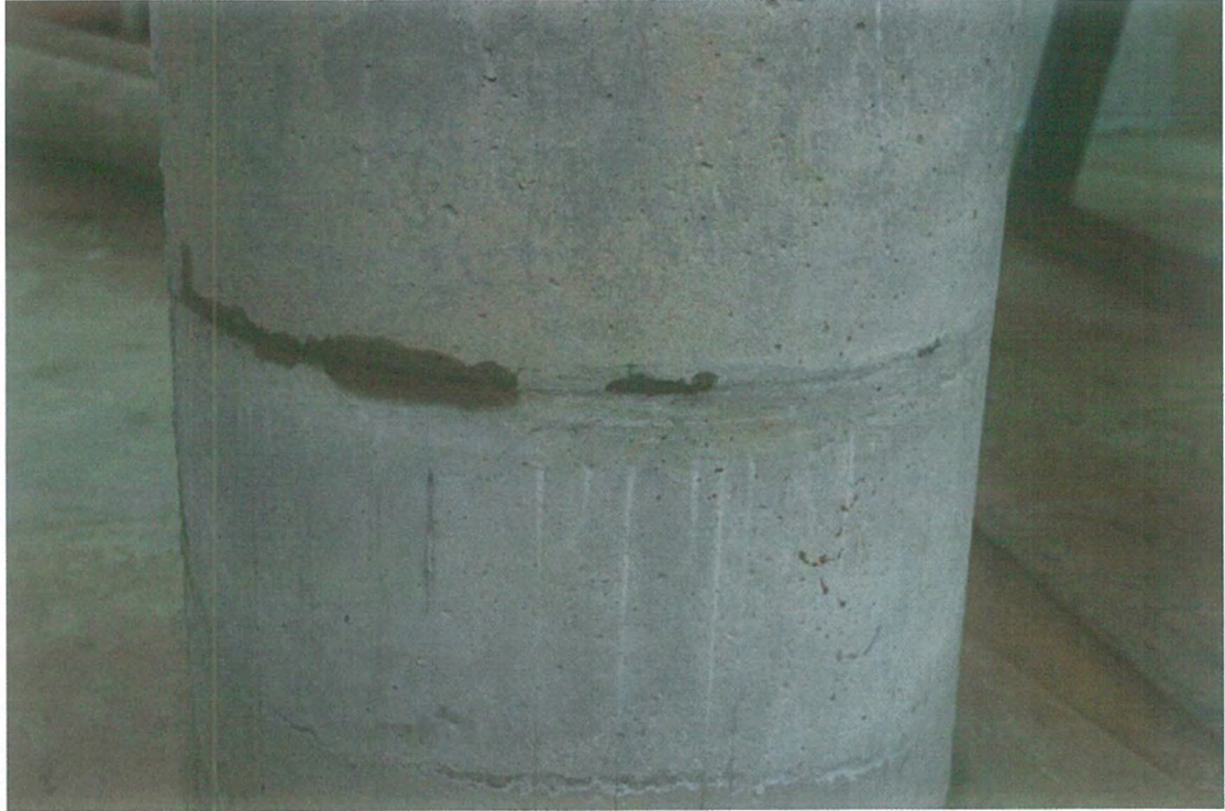
Photograph 5 – Increased leakage along the construction joint at 160 psi (112.7 m water) pressure.
