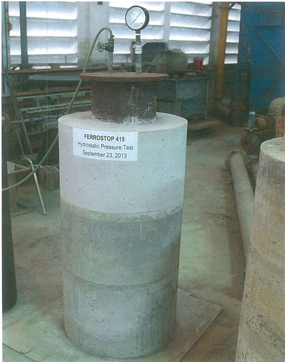
Photograph 3 – Concrete test chamber with 140 psi (98.6 m water) pressure. No leakage along the construction joints were noted.
