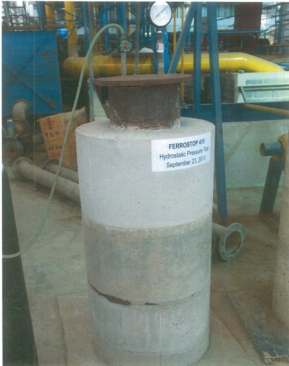
Photograph 4 – Concrete test chamber with 150 psi (105.6 m water) pressure. Initial Leakage occur along construction joint 1.
